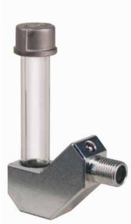
The Vista Zero offers outstanding all-round visibility and a compact design. The clever design sets the view level 12mm lower as on the normal typ level gauge type Vista. The sight glass, made of 3mm thick acrylic PMMA, is fixed tight into its metallic socket in a special process without additional bonding materials. As a result the product is more rigid than conventional products made of a brass/glass combinations with a 360° visibility. The display range is according to DIN3018.
